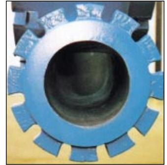
Shoulders, beveled fits and other contoured surfaces were reconstructed to original form with proper clearances.
